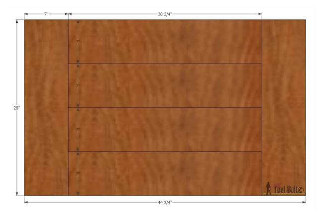
Cut the top pieces, 4 @ 30 3/4" and 2 @ 28". When using 2 x 8 for tops, I like to trim down the sides with a table saw to get a straight edge. The widths of the 2x8's are trimmed down to 7" wide.
