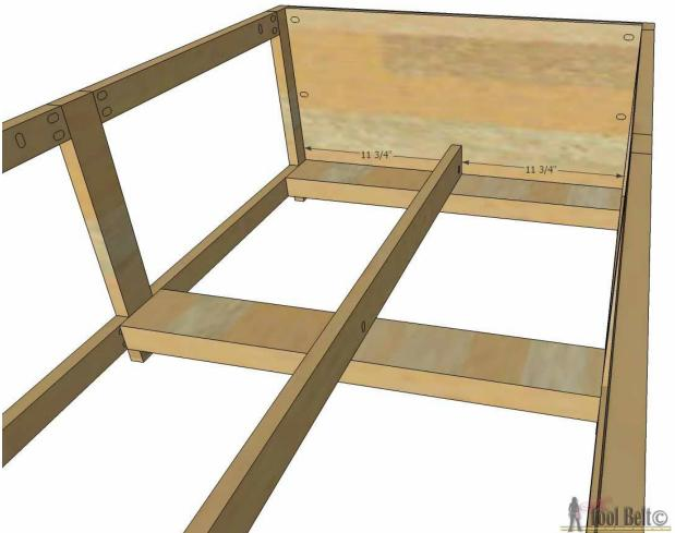
On the inside of the table, measure and mark on the supports from the inside face frame 11 <sup>3</sup>/<sub>4</sub>. Dryfit center divider and trim as necessary. Add 3 or so pocket holes in the center divider to attach it to the bottom supports. Use 1 <sup>1</sup>/<sub>4</sub>" screws to attach the center divider to the supports. The center divider is the backstop for the crates.
